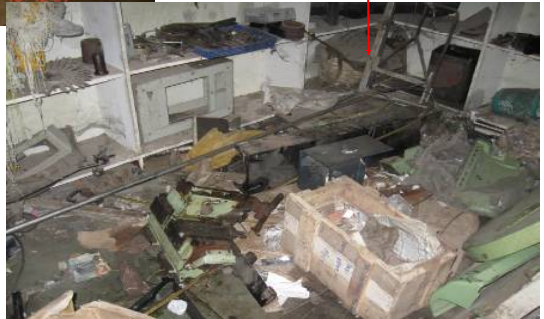
No protection to prevent damage and rust
